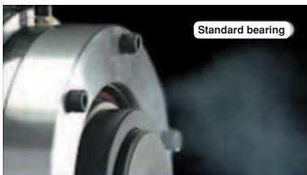
A large amount of oil mist passes through the bearing, contaminating the working environment.
