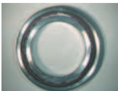
Photo. 6.1 Filling grease into angular contact ball bearing
