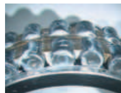
Photo. 6.2 Filling grease into cylindrical roller bearing
